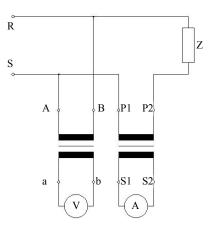
Figure 1: Connection of instrument transformers to the network.
